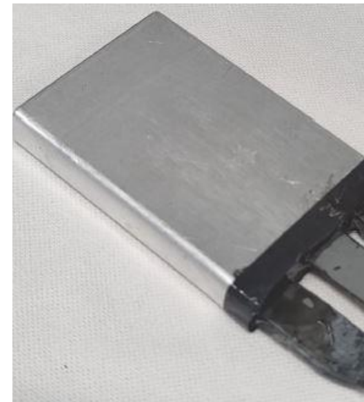
Left: Canned capacitor with 32 \mu F Right: Top view of encapsulated cap with XRT
