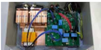
WBG converter prototype for the transmitter coil of a wireless charger while driving.
