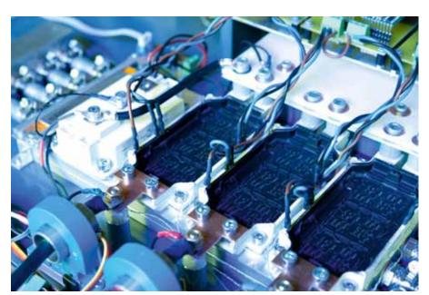
Experiment to analyse the thermal behaviour of the power semiconductors in an automotive traction inverter
