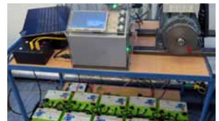
An integrated on-board battery charger for EVs based on nine-phase power electronics and propulsion motor.
