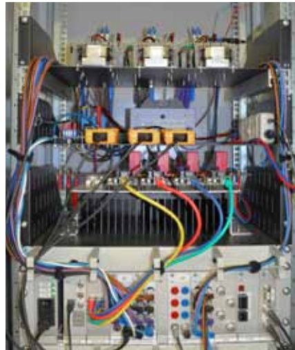
Teststand for an inverter with active neutral for unbalanced power infeed
