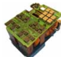
2 KW Power converter with embedded GaN semiconductors
